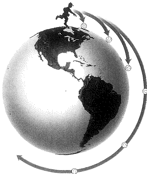
FIGURE 21 Satellite Motion The faster a projectile is thrown, the farther it travels before it hits the ground. A projectile with enough velocity moves in a circular orbit. Interpreting Diagrams How does the direction of gravity compare to the direction of the orbiting projectile's motion at any point?
