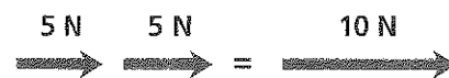
FIGURE 2 Combining Forces The strength and direction of the individual forces determine the net force. Calculating How do you find the net force when two forces act in opposite directions?
