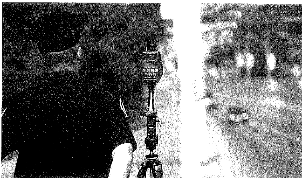
FIGURE 4 Radar Gun Radio waves and the Doppler effect are used to find the speeds of moving vehicles.
